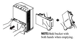
**Important:** Do not use the hose if using the water tank to collect water. When the hose is connected, water will be drained out through it onto floor instead of into the tank.
